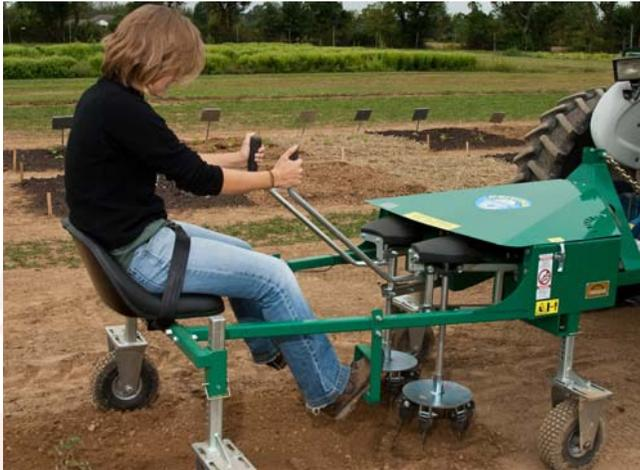
A participant demonstrates an Eco-weeder, a 3-point hitch, power take-off, driven tractor-mounted cultivator tool for removing weeds between plants laid out in a row
